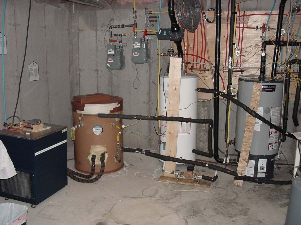
Figure 3: DWHR test setup
