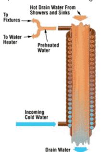
The GFX has a number of advantages for wastewater heat recovery:
