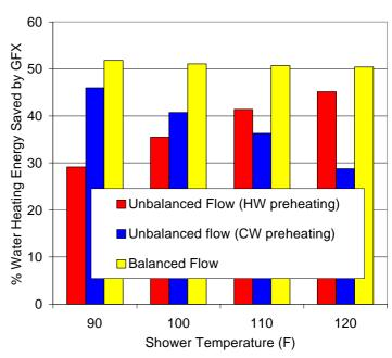
to preheat water to the water heater (HW preheating) is a reasonable option. Further, there would be no tempering of the cold water delivered to the fixtures in the dwelling.
